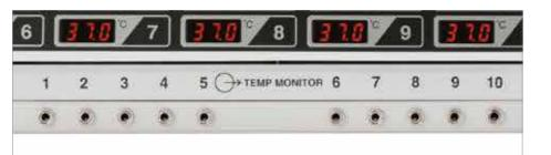
Equipped with an external temperature measurement jack for Quality Control (QC) measurements.
