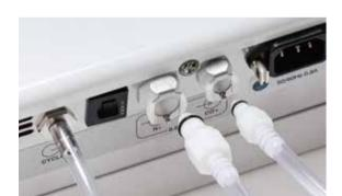
Standard quick-release connectors help to prevent incorrect connection of the CO<sub>2</sub>/O<sub>2</sub> tubing.
