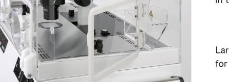
Large Side-doors on both sides for comfortable In-Out of Materials
