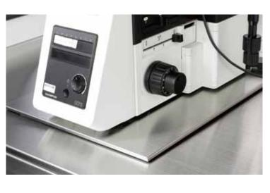
Built-in anti-vibration table comes with the workstation as a standard feature on AIM and AIMT models.
