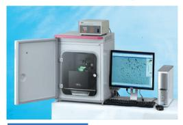
Microscope now rests in incubator under the condition of temperature 37°C and humidity >96%. Long-term observation of cultured cell is now possible without moving or sampling cells.
